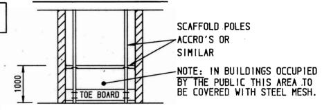
SAFETY BARRIER ARRANGEMENT TO SUIT AN ENCLOSED AREA IN FRONT OF LIFT WELL
