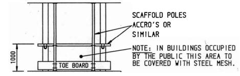
SAFETY BARRIER ARRANGEMENT TO SUIT AN OPEN AREA IN FRONT OF LIFT WELL
